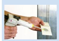
Apply sufficient Isomark compound to shiny side of the ID Sheet (opposite side to red printed half)
