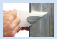
Allow Isomark compound to cure. Use the ID Sheet to carefully peel off the impression.
