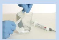
Allow Isomark compound to cure. Use the ID Sheet to carefully peel off the impression.
