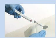
Apply sufficient Isomark compound to shiny side of ID Sheet (opposite side to red printed half)
