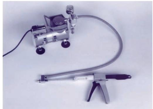
Compound XF Black is made up of two components (base and catalyst) which are contained within a cartridge. These two components are mixed during dispensing via a nozzle using a hand-operated gun dispenser. The resulting replicas have high resolution, are strong, flexible, dimensionally stable and highly opaque.
