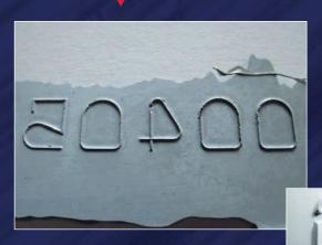
Magnified images of Isomark replica showing unique detail associated with the stamping tool
